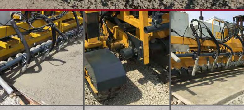
Integral vibrator and auger system to spread and consolidate concrete - reducing manpower needed in front of the paver.
